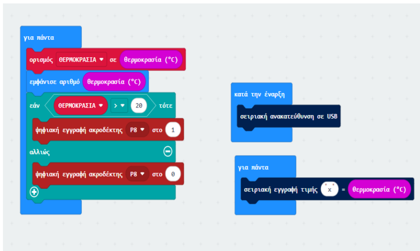
Figure 8. The code that took the temperature data and turned on the hazard light .
